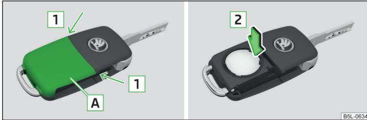
Fig. 184 Remove cover/take out battery
