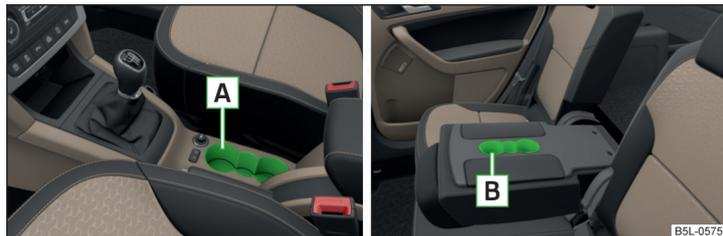
Fig. 78 Cup holders: in the center console, front / on the folding table in the center backrest
