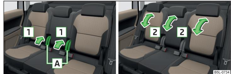
Fig. 68 Adjusting the seat backrest
