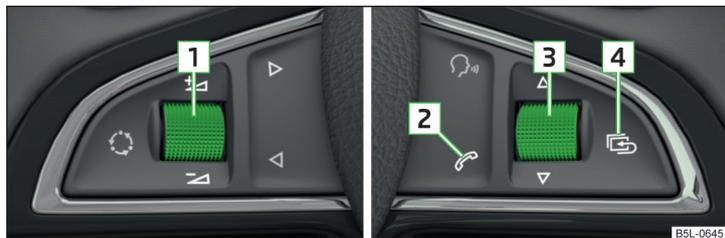
Fig. 118 Multifunction steering wheel: Control buttons for the telephone
