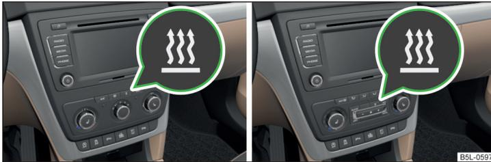
Fig. 114 Button for switching on/off the system directly on the operating part of the air conditioning/Climatronic
