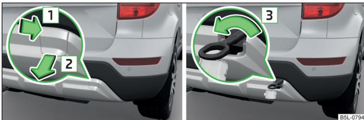
Fig. 183 Removing the cap / fitting the towing eye
