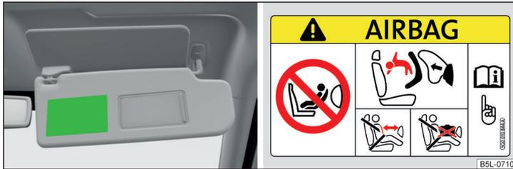
Fig. 17 Front passenger sun visor / label
