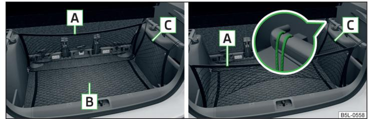
Fig. 96 Fastening examples for nets
