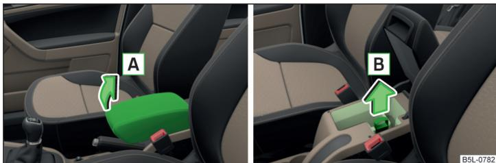
Fig. 85 Open storage compartment / open air supply
