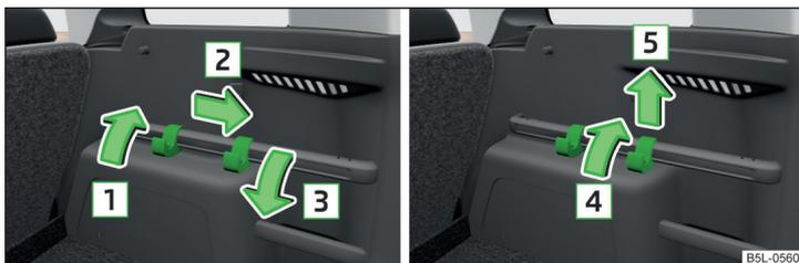
Fig. 98 Sliding hook on the mounting bar / removing hook
