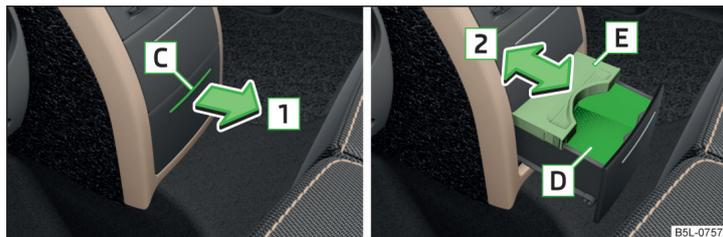
Fig. 79 Open cup holder in the central console / adjust holder size
