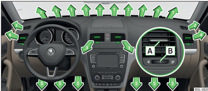
Fig. 109 Air vents at the front
