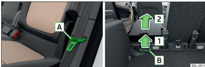
Fig. 69 Safety position of seat belt / folding the seat completely forward
