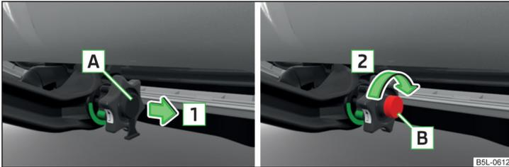
Fig. 153 Removing the lock cover/releasing the lock
