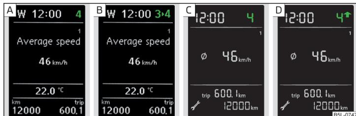
Fig. 29 Information on the selected gear / Gear recommendation
