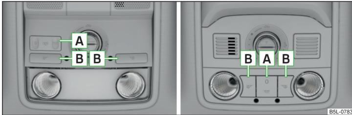
Fig. 51 Operation of the front light: Version 1/version 2
