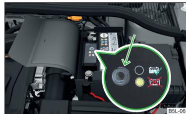
Fig. 165 Electrolyte level indicator
