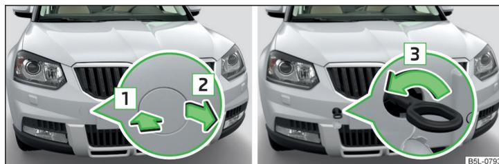
Fig. 182 Removing the cap / fitting the towing eye
