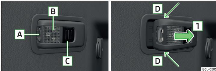
Fig. 104 Light operation / removal
