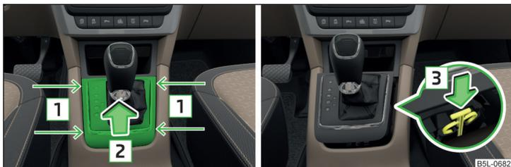
Fig. 190 Selector lever-emergency unlocking
